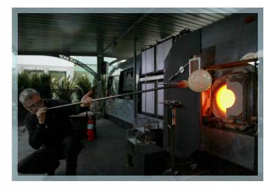
ABOVE, FROM LEFT: Paul Cunningham, Hot Shop supervisor, places a piece of glass into the glory hole to stabilize the heat of the piece before adding more color to the glass. Next, he shapes the hot glass using a forming tool made of cherry wood to ensure a smooth, even shape, and then blows into the blowpipe to inflate the size of the glass piece.
